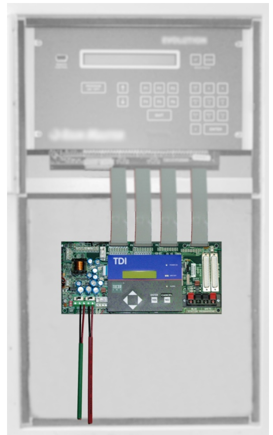
The TDI as installed in a conventional controller's cabinet
