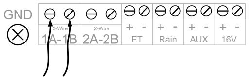
There's room for connecting two cables directly to the controller - the other line can be connected to the terminals labeled 2A-2B. Both wires will receive the same signals when the controller is up and running.
