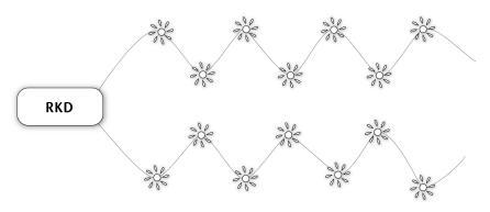
In contrast, this is how the above system would look using a conventional irrigation system that needs a dedicated cable to each individual valve:
