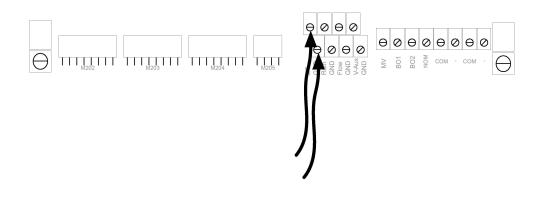
**Important!** Be aware of the polarity when you connect devices to the RKS+: Connect plus to plus and minus to minus or you won't see the expected behavior from the connected devices.
