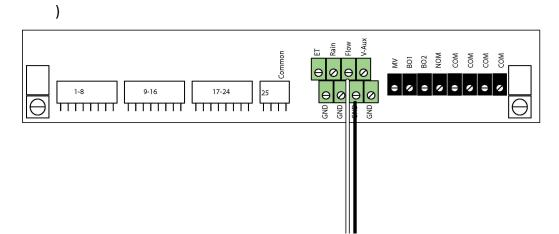
A photo diode type flow sensor is also connected to the "Flow" terminal, and via the "V-Aux" terminal through a resistor.
